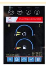
Remote Diagnosis: according to the real-time applications, shown on the centralized diagnos tic monitor, determine the location of the faults that may occur remotely.
